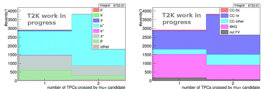
**Figure 4:** Events with  $\mu^+$  candidate crossing one (left bin) or two TPC chambers (right bin). Left plot: Colors indicate the true particle selected as  $\mu^+$  candidate. Right plot: Colors indicate the true topology of the event.
