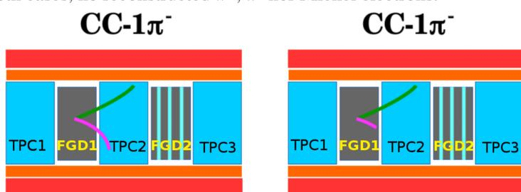
**Figure 2:** CC1 $\pi^-$  topology event in the ND280 tracker. Left:  $\pi^-$  candidate containing a segment in TPC. Right: with an isolated track in FGD1 interpreted as  $\pi^-$ .
