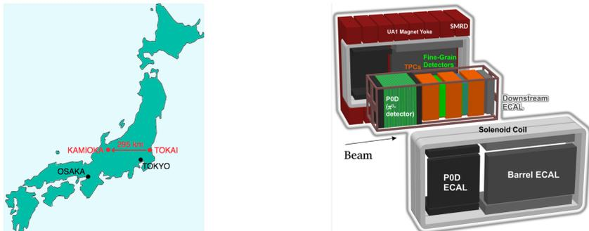
**Figure 1:** Left: Location of T2K experimental sites. Right: Cut-away drawing showing sub-detectors of ND280.
