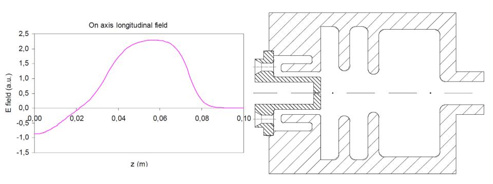
Cross Section: overall length 100 mm, maximum inner radius  $\approx 40$  mm
