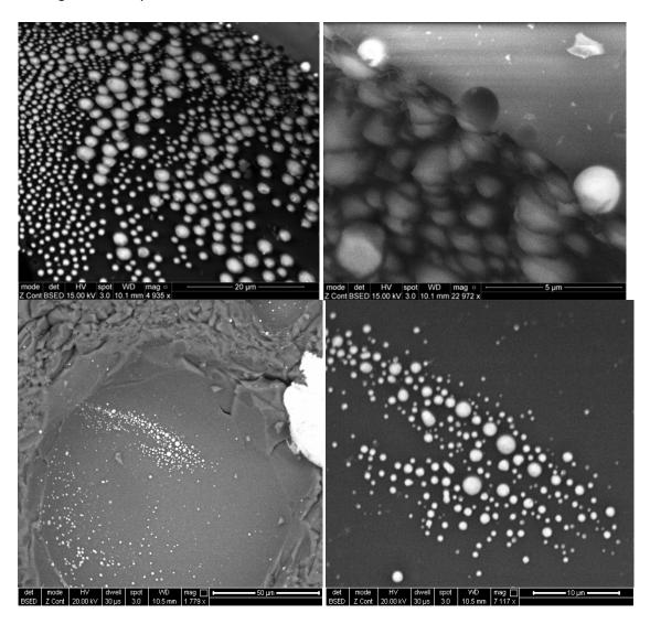
Upper left: A bimodal distribution of metal spheres (showing bright in the backscatter mode) decorating the inside of a vesicle. Upper Right: Detail of vesicle/glass transition showing spheres embedded in the glass and the imprint of a sphere that has been removed from its embedded position. Lower left: Vesicle exhibiting correlated and random deposition of metal spheres. Lower right: detail of correlated deposit.
