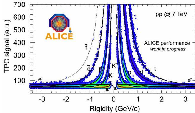
Figure 3: The  $dE/dx$ -spectrum for 7 TeV data.
