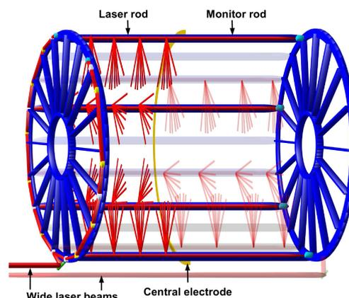
Figure 2: The laser calibration system.
