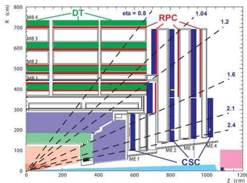
Figure 1: Layout of the CMS muon system.
