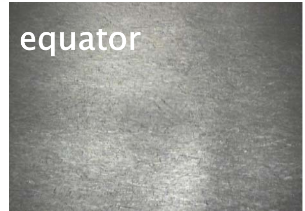
Large grain cavity after CBP
