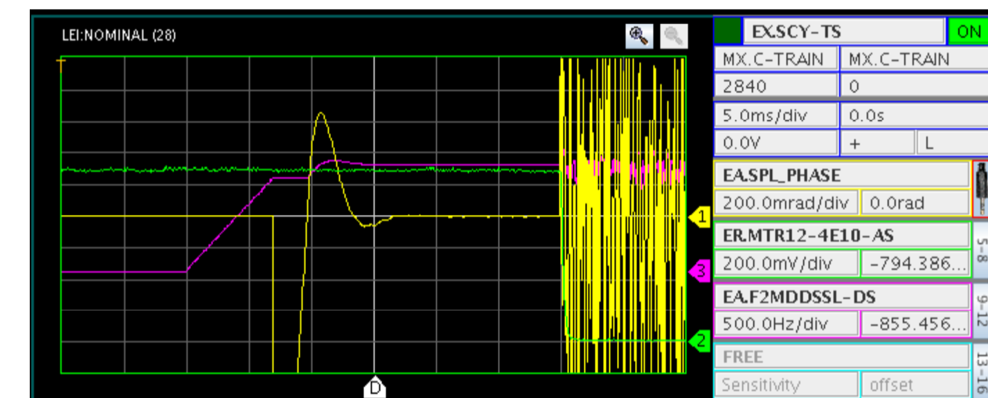
Analog and digital signals displayed together on the same virtual scope, triggered by the Start Cycle timing (EX.SCY-TS) with a trigger delay of 2840 ms.
