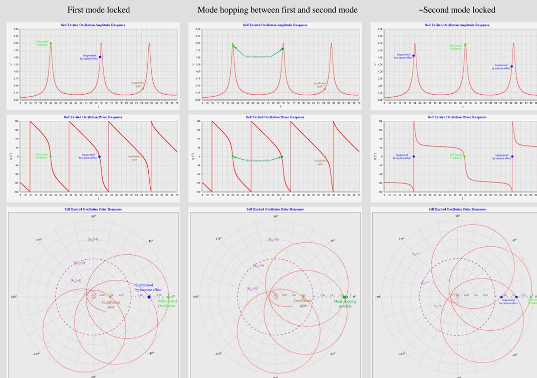
Using a fixed LO frequency of 1160MHz and varying the loop phase alone, we have been able to lock to 3 different cavity modes.
