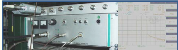
The TWT and the driver amplifier receive the "gate" signal from dedicated timing units. The driver can also be remotely controlled: in this way, via software, it is possible to change the power level of the whole RF chain for manual operation or for automatic conditioning of the klystron and the RF network first and the CLIC prototype accelerating structures, second.
