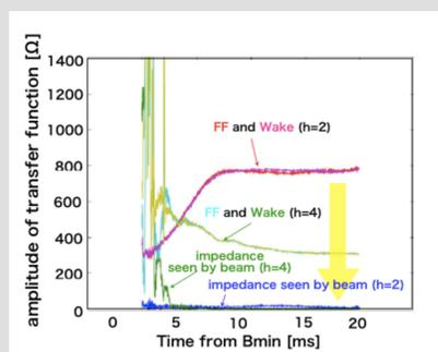
Comparison of the feedforward transfer function and the impedance seen by the beam, in the case of with and without feedforward. The impedance seen by the beam is kept less than  $25\Omega$  during the whole acceleration period.
