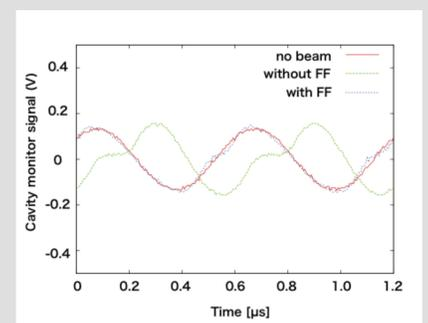
Comparison of the cavity voltage monitor waveforms just before extraction, in the case of no beam, without feedforward and with feedforward. The beam intensity is 300 kW equivalent. The waveform distortion and delay are reduced with feedforward.
