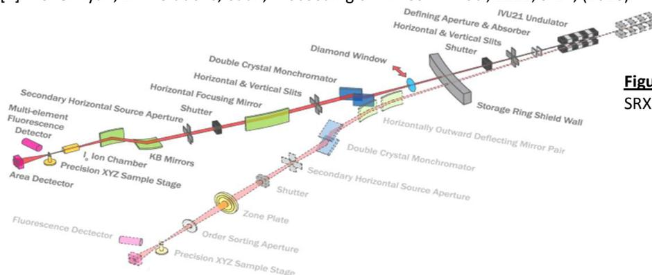
**Figure 1:** Optical layout of SRX beamline.
