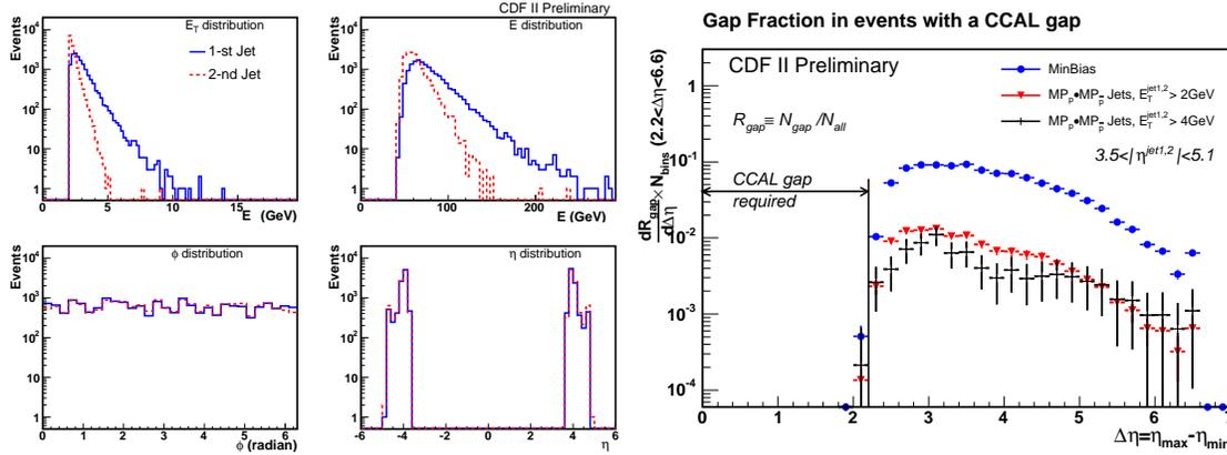
Fig. 3: (left) Kinematic distributions for the two leading jets in an event, both in the MP calorimeters. (right) The gap fraction  $R_{gap}$  vs.  $\Delta\eta$  for min-bias and MP dijet events of  $E_T^{jet1,2} > 2$  GeV and  $E_T^{jet1,2} > 4$  GeV.
