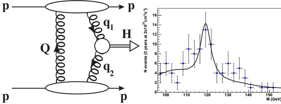
Fig. 3: (Left) Diagram for the CEP process; (Right) A typical mass fit for 3 years of data taking at  $2 \times 10^{33} \text{ cm}^{-2} \text{ s}^{-1}$  ( $60 \text{ fb}^{-1}$ ). The significance of the fit is  $3.5\sigma$  and uses only events with both protons tagged at 420m.
